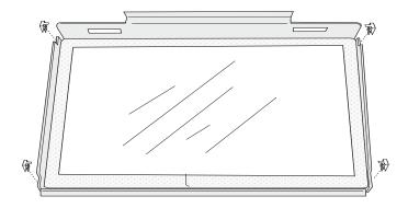
Figure 31. Use small pliers to pry up the two retainer tabs.
